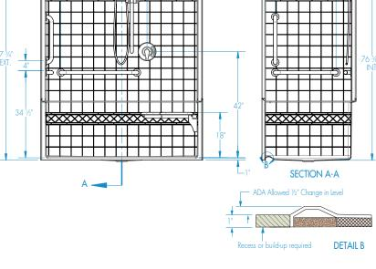
FEATURES Dimensional Tolerance ± %". Dimensions needed for site preparation should be measured from the unit. Aquatic assumes no responsibility for preparatory work.
