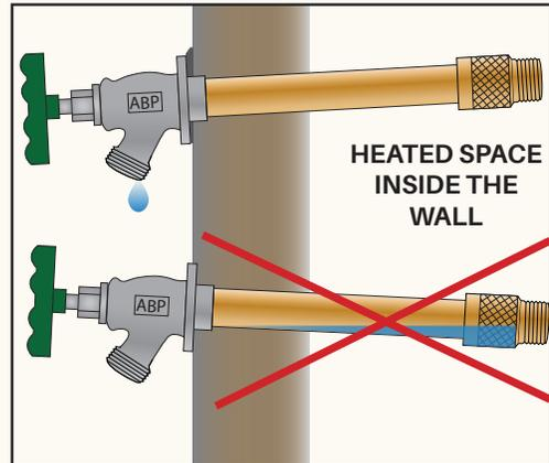
The only cause of a burst frost-proof hydrant is water expansion from freezing water inside an un-drained wall hydrant. Properly installed valves (with downward tilt) will always drain unless a hose or other device was left attached.
