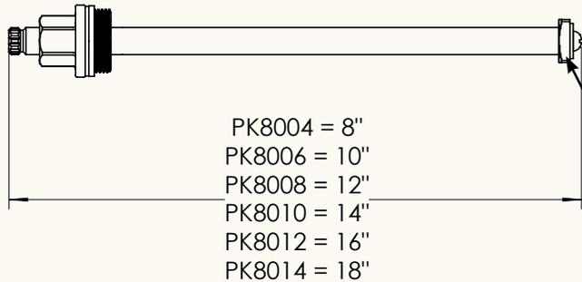
On faucets older than 1999: replacement stems may require a trim to the brass square washer retainer. Use a file or grinder to trim 1/16" off each corner to fit the stem into faucet. Contact Arrowhead Brass for more information.
