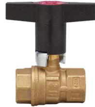
The NA108 series have an extended stem which allows operation if the valve body gets insulated. There is no need to purchase an expensive separate stem extension which then has to be field-installed between the valve body and handle. The valve features a blowout proof stem, PTFE seats, double o-ring stem seals, lead free brass ball and stem, and polyamide thermal plastic T handle.
