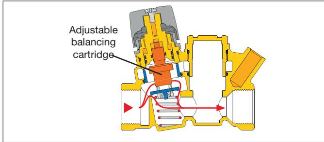
Optional check valve are available for all models, which protect against circuit thermo-syphoning.
