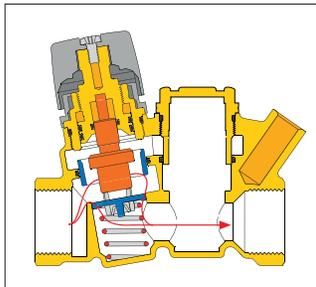
**Operating mode B - Automatic thermostatic disinfection**
