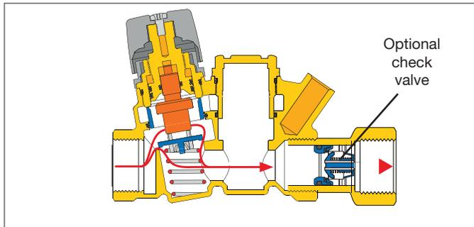
For systems using thermal disinfection for Legionella growth protection, the 1162xx series models incorporate a second thermostatic by-pass cartridge that activates at 160°F. The 1166xx series models activates at 140°F. A second flow path opens providing flow for the disinfection process which is independent of the primary balancing cartridge.
