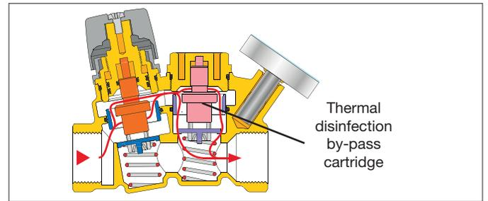
Alternately, the 1163xx series models incorporate a by-pass valve for thermal disinfection which is activated by an optional field mounted thermo-electric actuator, code 656 series, controlled by an automation system.
