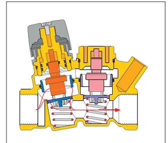
**Operating mode C - Actuator-controlled disinfection**
