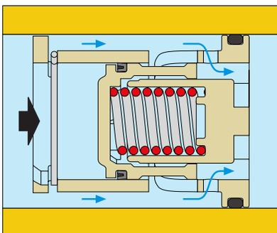
In this case, the spring-loaded piston fully compresses a spring and leaves only the fixed orifice for the fluid to pass through. The flow rate through the FlowCal depends only on the differential pressure.
