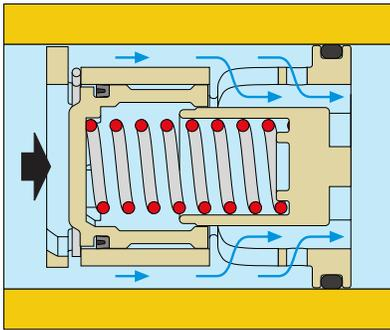
In this case, the spring-loaded regulating piston remains in equilibrium without compressing the spring and gives the fluid the maximum free flow area. When below the differential pressure control range the piston acts as a fixed orifice and thus the flow rate through the FlowCal depends only on the differential pressure.
