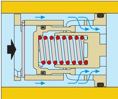
If the differential pressure is within the control range, the spring-loaded piston is positioned to give the fluid a free flow area permitting regular flow at the **nominal rate** for which the FlowCal is set up.
