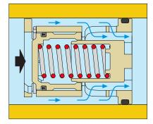
In this case, the spring-loaded regulating piston remains in equilibrium without compressing the spring and gives the fluid the maximum free flow area. When below the differential pressure control range the piston acts as a fixed orifice and thus the flow rate through the FlowCal depends only on the differential pressure.
