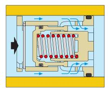
If the differential pressure is within the control range, the spring-loaded piston is positioned to give the fluid a free flow area permiting regular flow at the **nominal rate** for which the FlowCal is set up.
