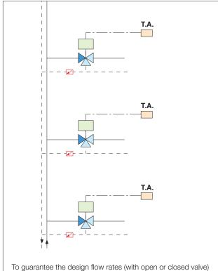
To guarantee the design flow rates (with open or closed valve) to the various zones of a system.
