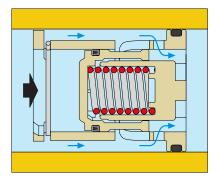
In this case, the spring-loaded piston fully compresses a spring and leaves only the fixed orifice for the fluid to pass through. The flow rate through the FlowCal depends only on the differential pressure.
