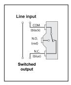
Flow switch used to activate a device when flow stops. When the decreasing operating flow is reached or stops the common (black wire) and the normally open (red wire) contacts open, while the common (black wire) and the normally closed (blue wire) contacts close.
