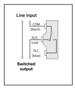
Flow switch is used to activate a device when flow starts. When flow starts and the increasing operating flow is reached or exceeded, the common (black wire) and normally open (red wire) contacts are closed, while the common (black wire) and the normally closed (blue wire) are open.
