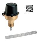
The Caleffi Series 626 water flow switch detects the presence or absence of flow in piping of heating, air conditioning, cooling and water treatment systems as well as in pumping and process systems. In heating systems, the flow switch is normally used to shut off the burner of the boiler whenever there is no circulation of the carrier fluid in the boiler circuit. A lack of circulation can damage critical components and impair the operation of temperature sensitive safety and protection devices.
