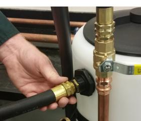
4) Connect opposite end of second hose to pump cart return at bulkhead fitting.
