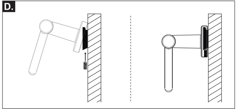
1. Attach Assist Bar onto mounting bracket and secure with the provided 10-24 X 1/2" Socket Set Screw. Repeat for opposing side.
