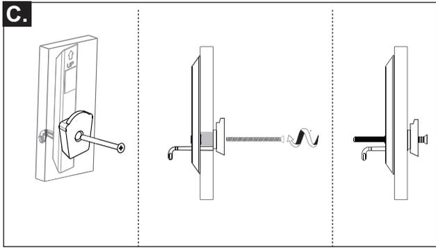
1. Hold on tightly to the flange and keep pressure on the bar behind the wall to ensure that the bar stays upright with the longest part of the bar pointing upward. The bar behind the wall must always be upright and the longest part must be pointing upward for the anchor to perform properly.
