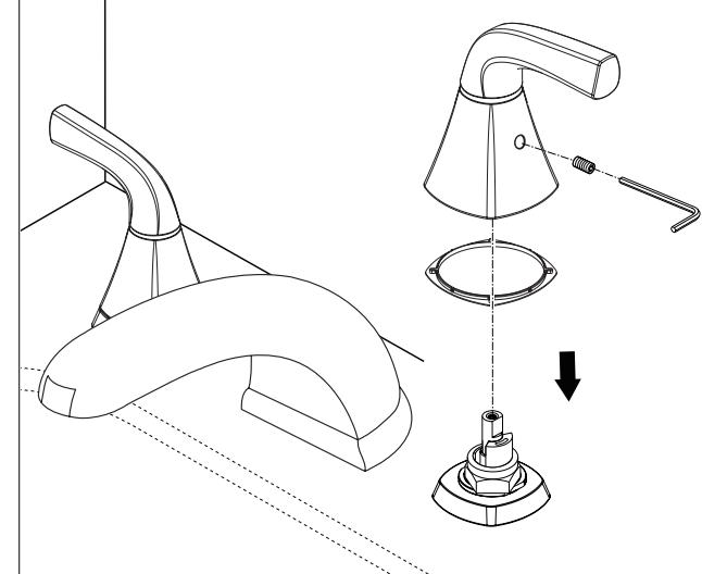
**NOTE: The deck and valve rough-in must be finished before installing the trim kit.**
