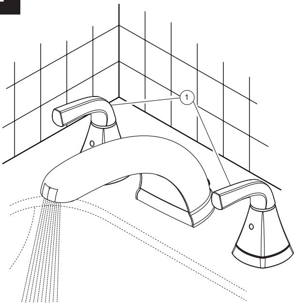
Turn faucet handles (1) all the way on. Turn on hot and cold water supplies and flush water lines for one minute.
