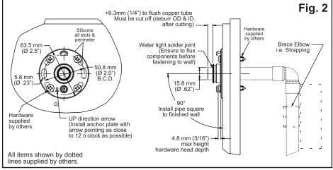
plate is being mounted to. The anchor plate slots are designed to suit 3/16" (4.8 mm) diameter fasteners. **Note:** The fastener head height can be a maximum of 3/16" (4.8 mm). Note the arrow on the anchor plate indicating the UP direction. Mark and drill the required holes for the hardware and anchors chosen (see Fig. 2). (Note: Mounting hardware is supplied by others.)
