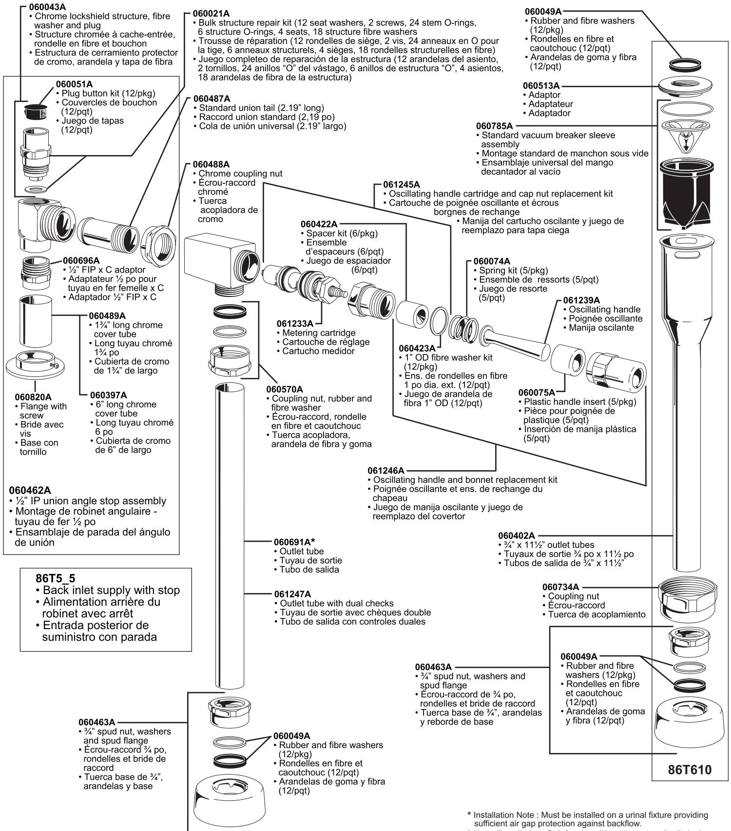
\* Installation Note : Must be installed on a urinal fixture providing sufficient air gap protection against backflow.
