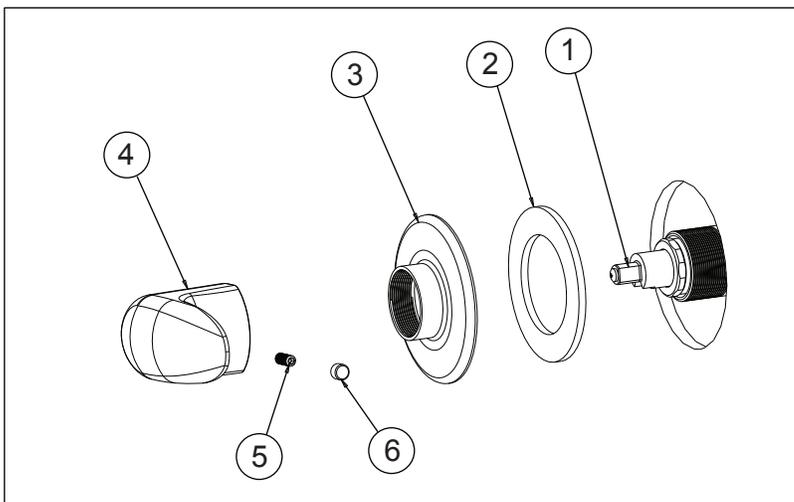
Put gasket (2) and escutcheon (3) over the extender. Attach handle (4) to the extender (1), they have a keyed fit. Secure the handle using the set screw (5) and cover the set screw with the button (6).
