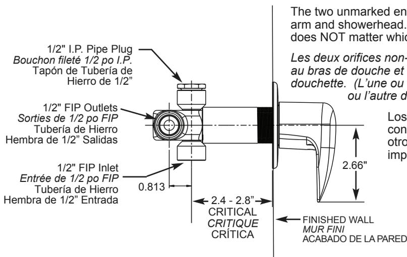
The two unmarked ends are OUTLETS: One is connected to the shower arm and showerhead. The other is connected to the handshower. (It does NOT matter which one goes where.)
