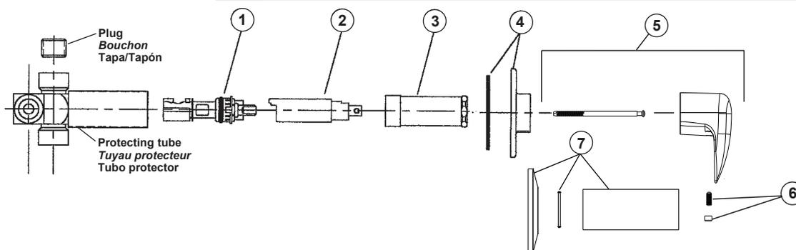
1/2" I.P. Plug is supplied to plug one of the "INLETS" (ONLY required one inlet - both inlets are marked "INLET" on body).
