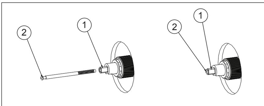
Thread handle screw (2) until it bottoms out in the the extender (1).
