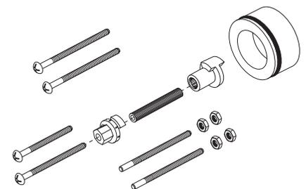
\*Depending on the location of valve within the wall and wall thickness an optional extension kit (RP72604) can provide an additional 1 3/4" of wall thickness.
