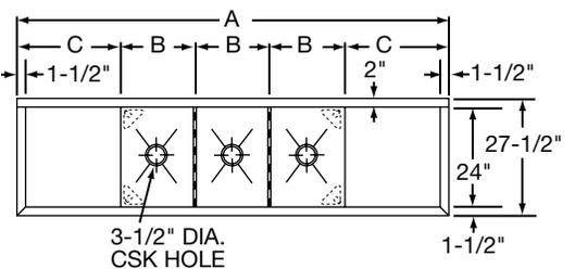
INDICATE NUMBER OF FAUCET HOLES WHEN PLACING ORDER. (NON-STANDARD FAUCET AND OVERFLOW DRILLING LOCATIONS ARE AVAILABLE. SPECIFY ON DRAWING AT RIGHT.)
