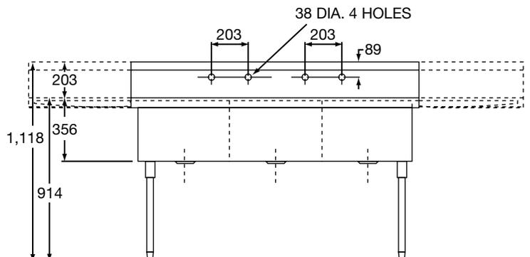
INDICATE NUMBER OF FAUCET HOLES WHEN PLACING ORDER. (NON-STANDARD FAUCET AND OVERFLOW DRILLING LOCATIONS ARE AVAILABLE. SPECIFY ON DRAWING AT RIGHT.)
