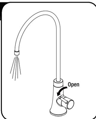
After installation is completed, turn on water supply, turn the handle in a counterclockwise direction. Flush the water lines for at least one minute. Important: This flushes away any debris that could cause damage to internal parts. Check for leaks.
