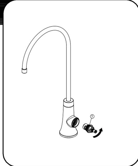
Loosen cartridge (1) by turning it counter-clockwise and lift it out. Insert new cartridge. Reinstall the handle.
