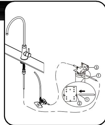
Connect the bottom of pipe (1) into the end (2) with outlet indicated of the filtration manifold (3). Pull moderately to ensure the connection has been made.
