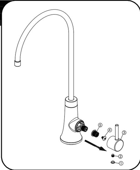
Shut off water supply. Remove index (1) and unscrew the set screw (2) on the handle (3). Remove handle (3) and loosen the screw (4) from valve stem. Loosen the inverter (5).
