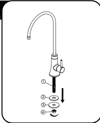
Before installation, shut off water supplies, remove old faucet. Remove the nut (4), metal washer (3) and rubber washer (2) from shank (1).
