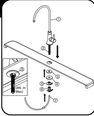
Place faucet (1) through the hole in countertop. Secure the faucet (1) to the countertop using the rubber washer (3) and the metal washer (4) provided. Tighten the nut (5), do not overtighten. Then tighten one end of the connector (6) joint at the bottom of the shank (2) and connect the other end to the pipe (7).
