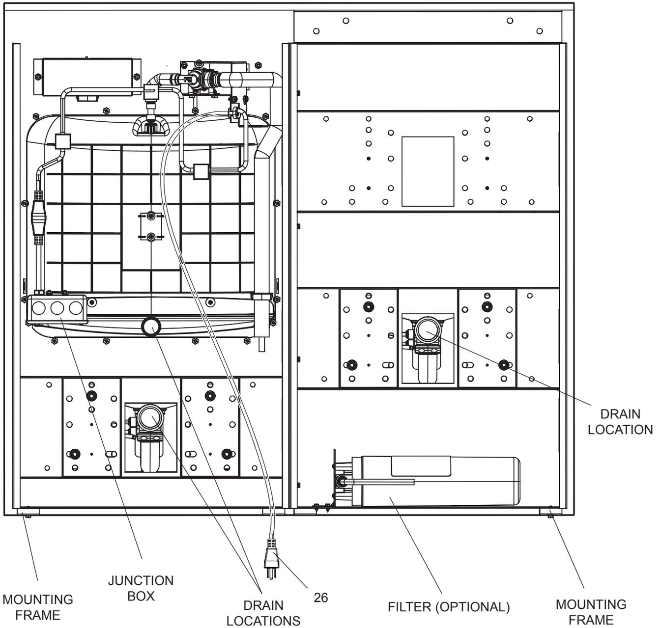
**NOTE:** Bottle filler back cover removed from the view for clarity
