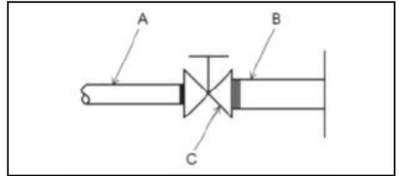
**LEGEND** A = 3/8" (9.5mm) O.D. Tube. Water Inlet to Chiller
