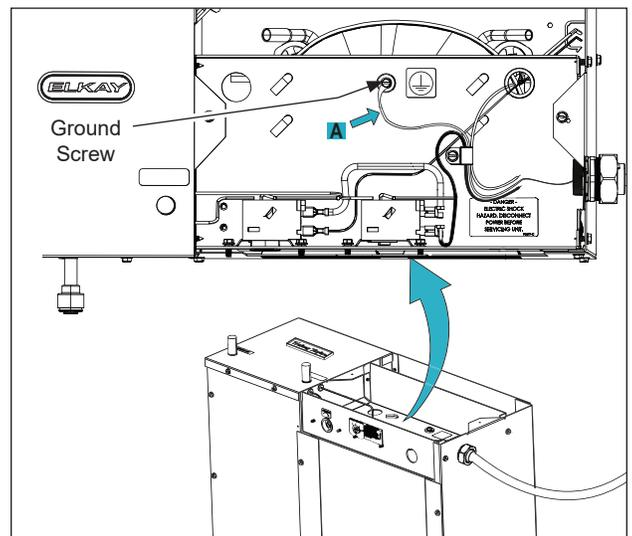
5. Connect the black wire (B) to supply voltage HOT and connect the white wire (C) to neutral line.
