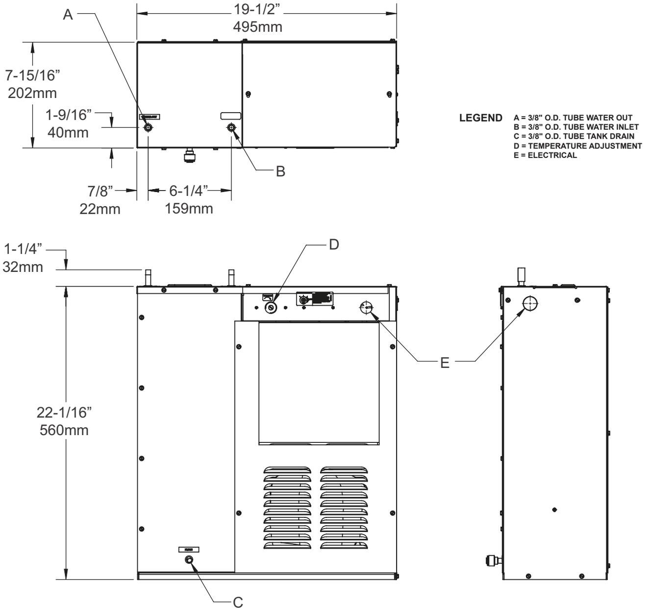
For remote installation a minimum clearance of 6 inches (152 mm) to the front must be maintained, 1 inch (25 mm) each side, 3 inches (76 mm) to the rear above the unit. Wall grille EG-1 or EG-2 to be used when unit is inserted into an enclosure. Install unit as close as possible to wall grille. A 6 inch (152 mm) clearance beyond the front of the wall grille is required for adequate air circulation.
