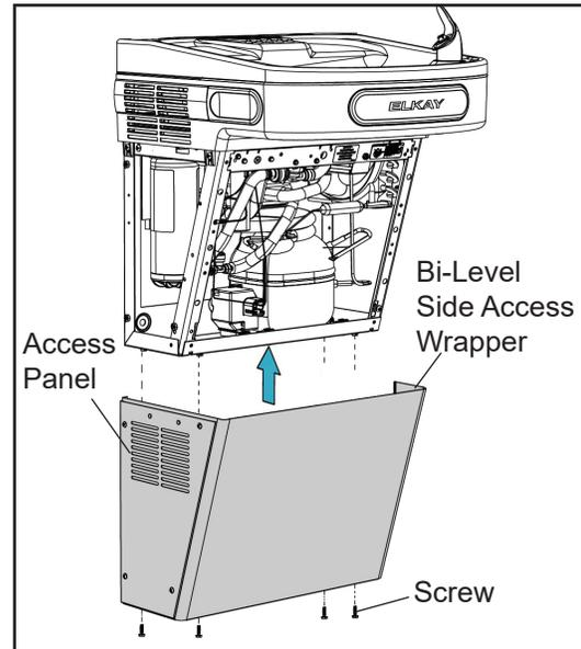
**Note:** While the side access wrapper is being secured, verify the upper profile (left, front, and right side) of the wrapper frame slides up and under the plastic basin shroud assembly for a tight fit (as shown).
