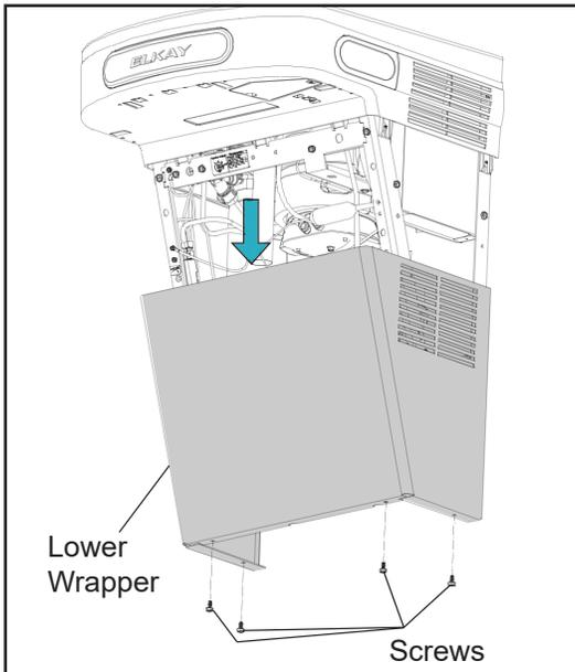
**Note:** While the side access wrapper is being secured, verify the upper profile (left, front, and right side) of the wrapper frame slides up and under the plastic basin shroud assembly for a tight fit (as shown).
