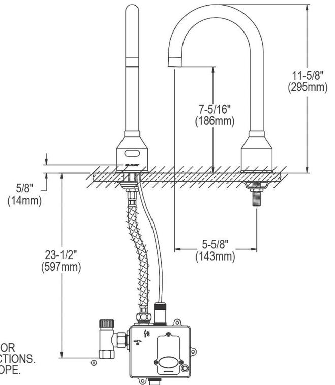
NOTE: USE TEFLON TAPE FOR ALL WATER CONNECTIONS. DO NOT USE PIPE DOPE.
