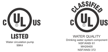
Fig. 4 Left: UL approval mark for water-circulation pumps. Right: UL approval mark for drinking-water system components made of stainless steel.
