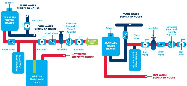
Not a warranty problem. Mini electric water heater tanks minimize cold water slugs.
