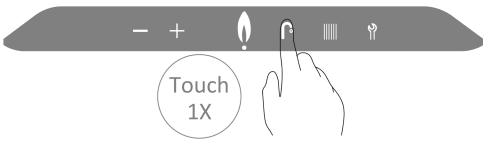
3. To change the DHW target temperature, touch the Plus or Minus buttons.
