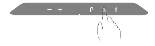
**3.** To change the space heating target temperature, touch the Plus or Minus buttons.
