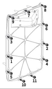
Figure 48: Tighten Allen bolts in cross pattern direction.
