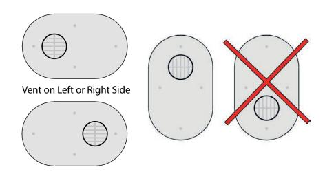
Figure 16 PVC low profile termination acceptable orientations
