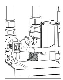
Figure 57: Domestic Hot Water Temperature Sensor S3
