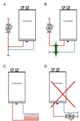
Figure 27: Permitted and prohibited space heating combi boiler piping
