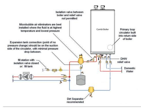
Figure 26: Boiler trim basic options – concept drawing is only a simple schematic guide
