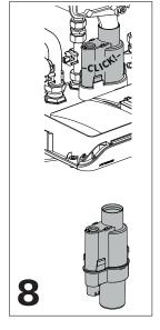
**14.** Slide the flexible hose onto the condensate trap base and into the drain (10)
