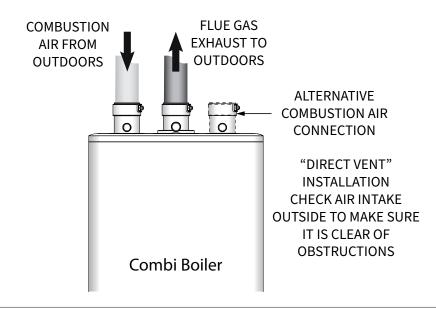
Figure 20: Direct vent combustion air intake
