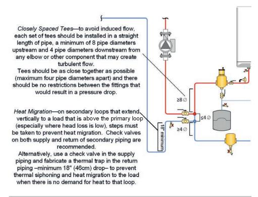
Figure 28: Basic Primary/Secondary piping with closely-spaced tees concept – concept drawing. This drawing is only a simple schematic guide.
