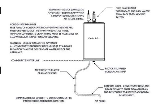
Figure 22: Condensate trap drainage
