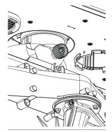
Figure 55: Flue Gas Temperature Sensor S5
