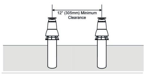
Figure 11: Vertical Concentric Termination - Two Kits
