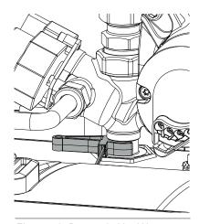
Figure 56: Domestic Hot Water Flow Sensor
