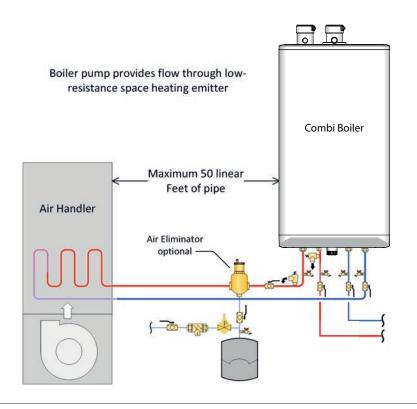
Figure 33: Air handler and direct domestic hot water – parallel piping for low loss heat emitter concept drawing. This drawing is only a simple schematic guide.
