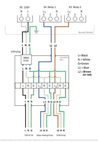
Figure 39: Junction box schematic
