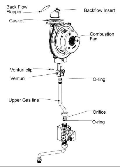
Figure 47: Blower and Gas Valve Assembly
