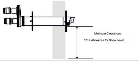
Figure 18: Horizontal Polypropylene Concentric Termination - Single Kit
