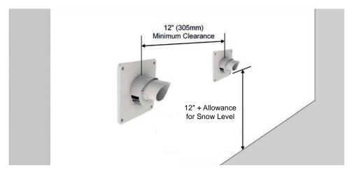
Figure 17: Horizontal Polypropylene Concentric Termination - Two Kits
