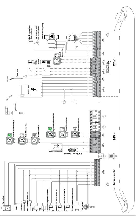
Diagram 6.2-3: Electrical wiring diagram
