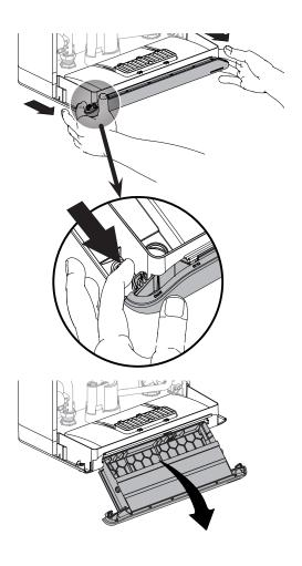
Figure 38: Pullling out the tray
