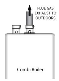
Figure 6: Basic exhaust vent assembly
