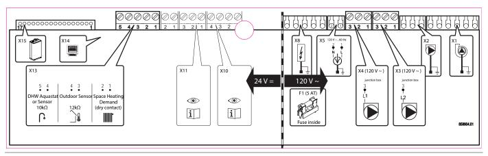
Figure 42: Terminal strip for connection of the DHW Aquastat (optional), thermostat or end switch(es) (mandatory), outdoor sensor (optional)
