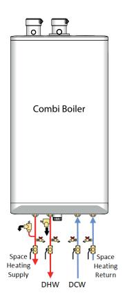
Figure 24: Overview of piping connections
