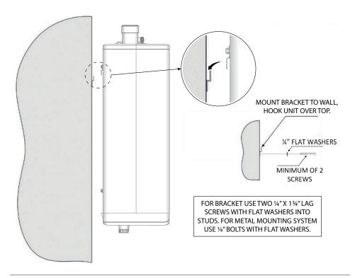
Figure 2: Wall mounting of unit
