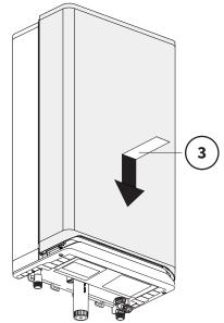
Figure 5: Positioning the frontpanel
