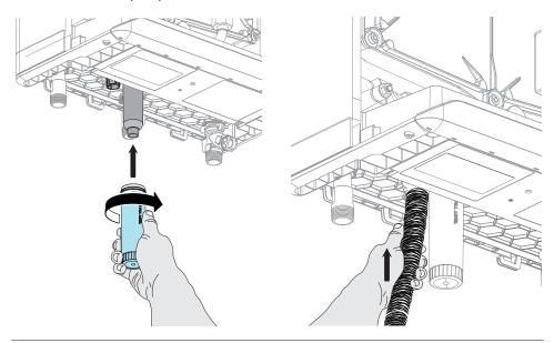
Figure 21: Condensate trap installation
