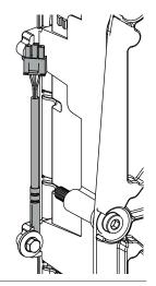
Figure 50: Heat exchanger Temperature Sensor S0
