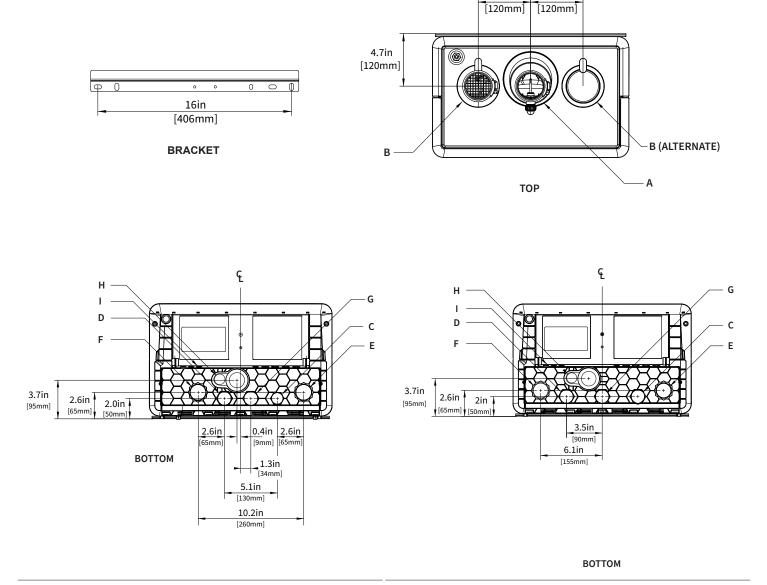
Figure 1b: Dimensions / Connections for Combi Boiler Models 99 - 125 Figure 1c: Dimensions / Connections for Combi Boiler Models 160 - 199
