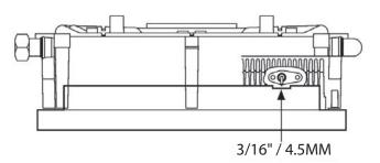
Figure 49: Checking igniter gap using 251-001 Ignitor Gapping Tool
