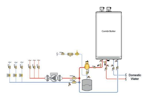
Figure 30: Typical one temperature space heating piping concept with direct domestic hot water – concept drawing. This drawing is only a simple schematic guide.
