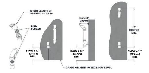
Figure 13: Sidewall vent termination - piping configuration
