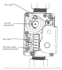
Figure 43 Gas Valve Adjust
