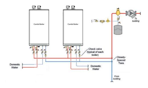
Figure 29: Multiple combi boiler piping concept – concept drawing. This drawing is only a simple schematic guide.
