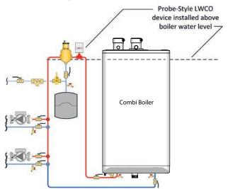
Figure 41: External Probe Type Low Water Cutoff Device
