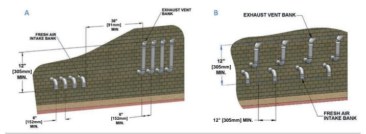
Figure 15: Sidewall vent termination - multiple vent piping configuration
