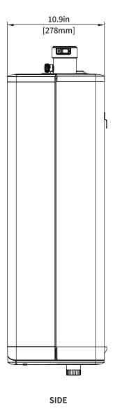
Figure 1a: Dimensions / Connections for Combi Boiler
