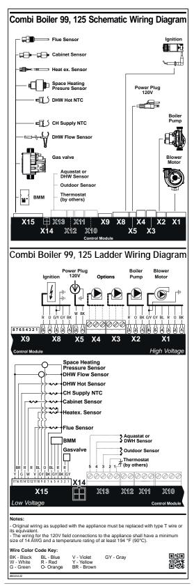
Diagram 6.2-1: Schematic wiring diagram 99 & 125 models
