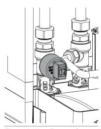
Figure 53: Water Pressure Sensor Type LWCO
