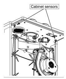
Figure 52: Cabinet Temperature Sensors
