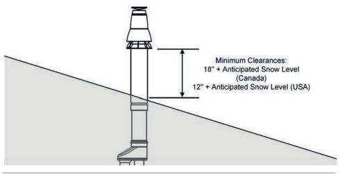
Figure 12: Vertical Concentric Termination - Single Kit
