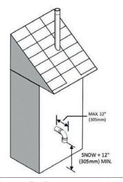
Figure 9: Rooftop vent terminal configurations
