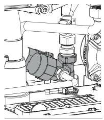
Figure 58: Domestic Hot Water Bypass Valve
