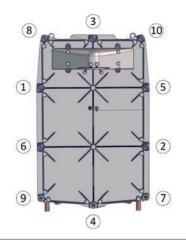
Figure 36: Tighten hex bolts in cross pattern direction.
