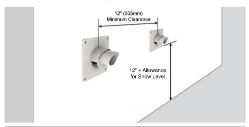
Figure 17: Horizontal Polypropylene Concentric Termination - Two Kits
