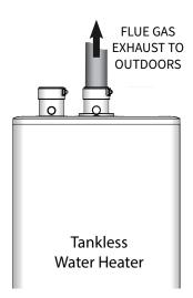
Figure 6: Basic exhaust vent assembly
