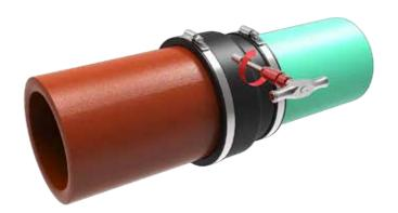
Tighten clamp bolts alternately and firmly to 60 in/lbs. of torque.
