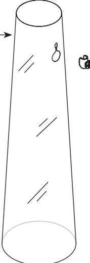
Isolates the pulldown hose from plumbing lines and other items under the kitchen sink.
