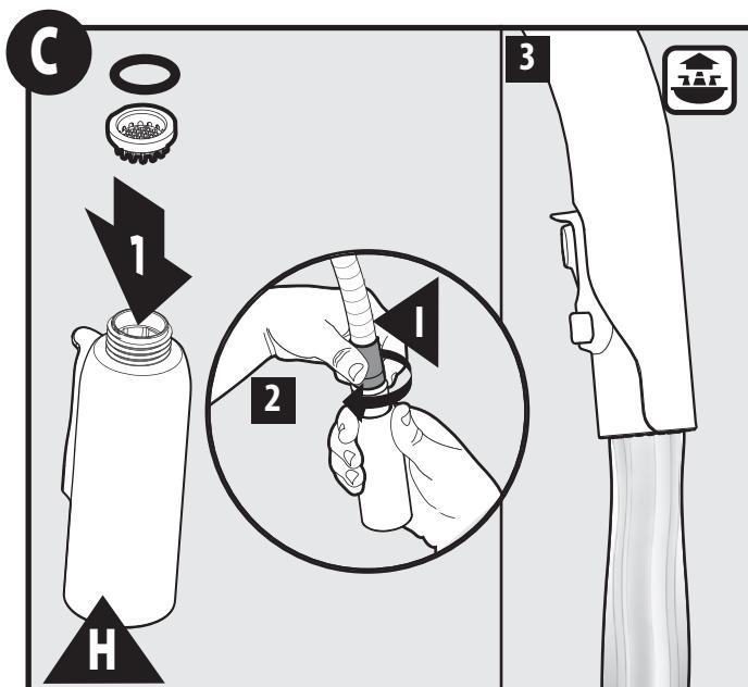
Reinstall screen and o-ring as shown. Thread Pulldown Hose (I) onto Spray Wand (H) and tighten as shown in frame 12. Re-check water flow.
