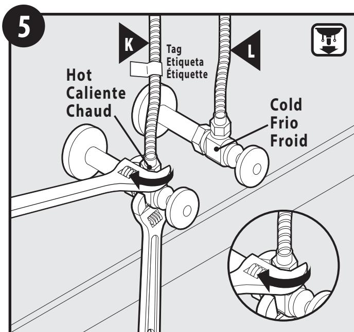
Connect hot (K) and cold (L) supply hoses to water supply valves.
