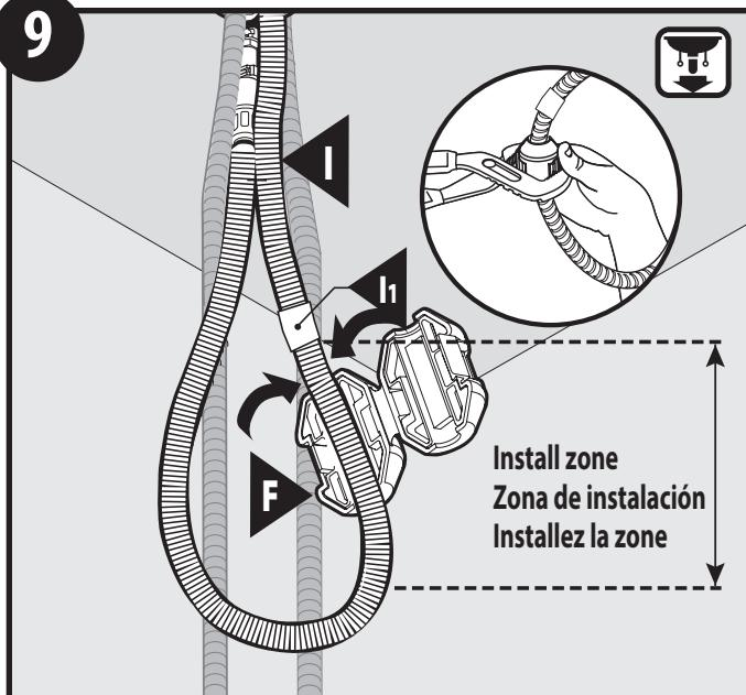
Remove and discard plastic cap from end of Pulldown Hose (I). Insert hose into end of Outlet Hose (J). Push until a "click" is heard. Tug downward to test engagement.
