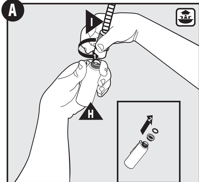
Unscrew Pulldown Hose (I) from Spray Wand (H) and remove screen and o-ring.
