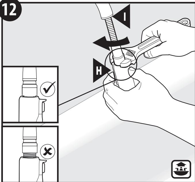
Tighten Pulldown Hose (I), flush with Spray Wand (H). Do not overtighten.
