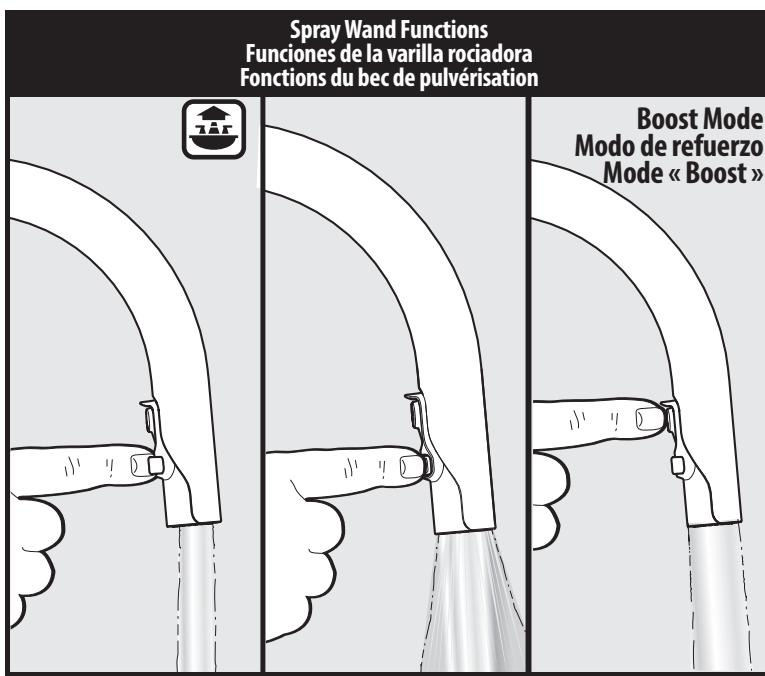
Check operation of spray wand. Turn on faucet, spray wand should be in stream mode. Push and release button on spray wand. The spray wand should change to spray mode. To enter PowerBoost™ mode, press top button. To exit the boost mode, turn off the faucet. **Note:** The spray wand will remain in the last used mode, once faucet is turned off. Manually choose your desired spray setting as faucet is turned back on.
