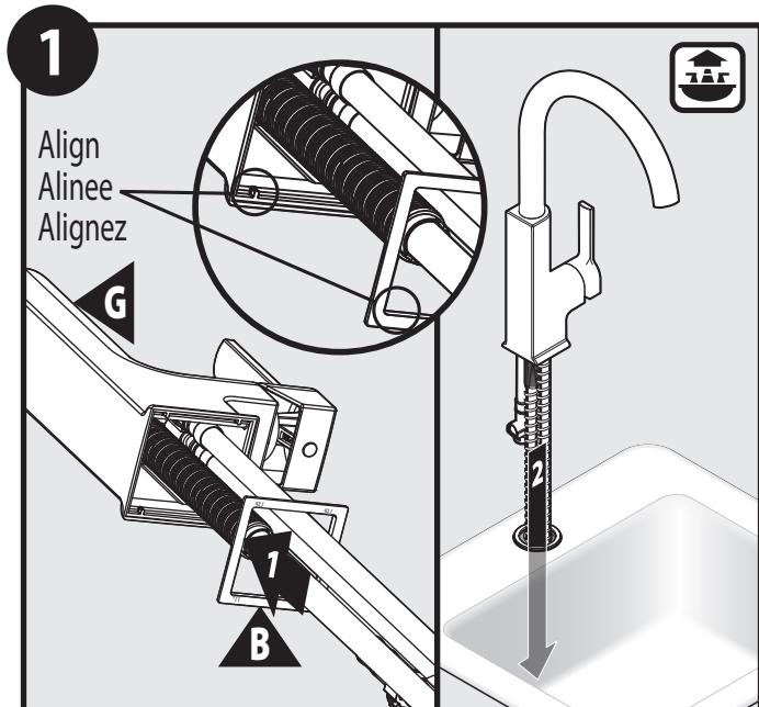
Place deck gasket (B) onto base of faucet body (G). Place into sink hole. **NOTE:** Install with handle on right side only.
