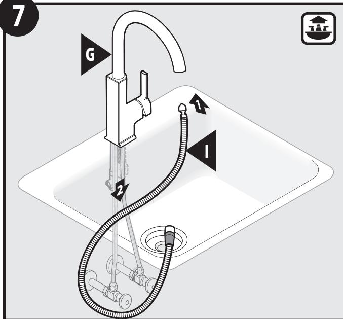
Slide hose swivel cover (M) onto Pulldown Hose (I). Push over swivel until cover snaps in place.
