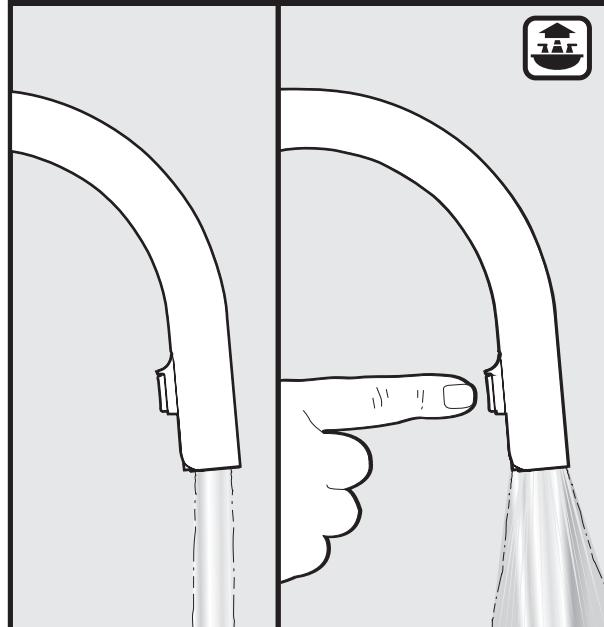
Check operation of spray wand. Turn on faucet, spray wand should be in stream mode. Push and release button on spray wand. The spray wand should change to spray mode. To switch back to stream mode, turn handle off and on again.
