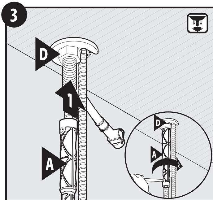
Tighten mounting nut (D) with installation tool (A). Use screwdriver through hole in installation tool (A) to tighten firmly.
