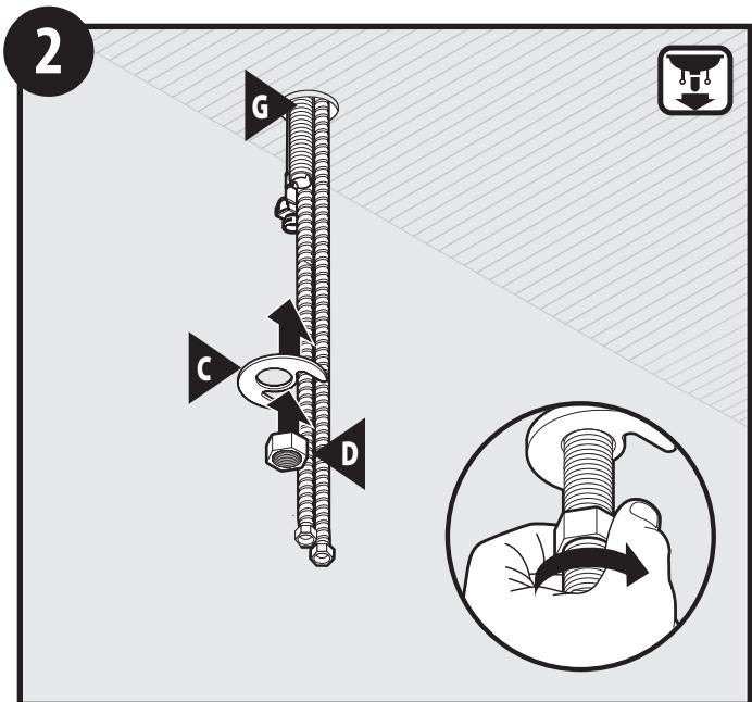
Slide mounting washer (C) up onto faucet body (G) under sink and secure with mounting nut (D).
