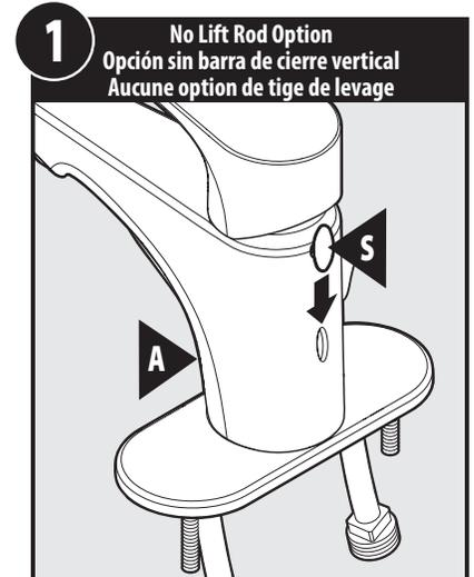
For Faucet installed without Lift Rod (L): Insert Plug Button (S) into slot in Faucet Body (A).
