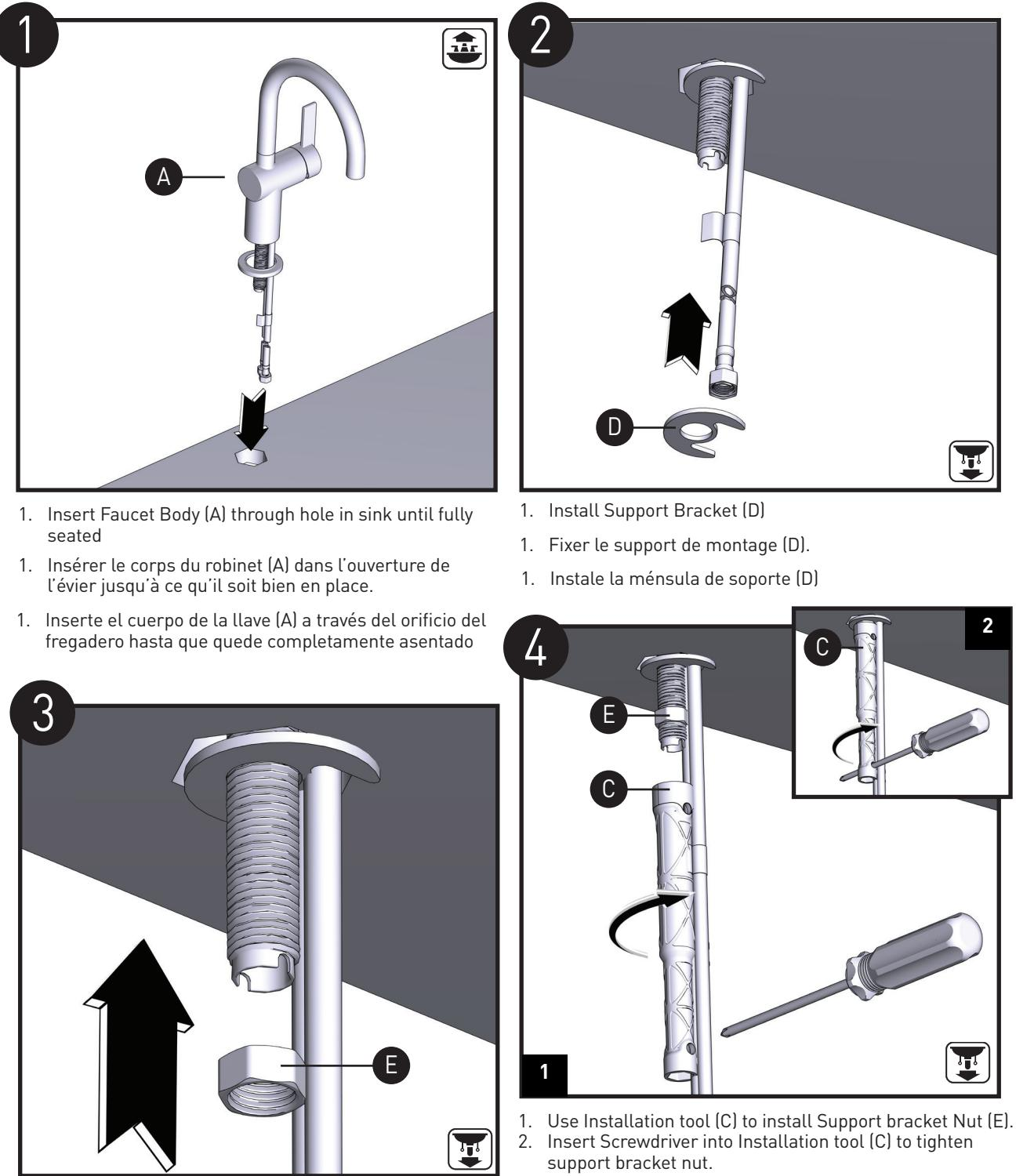
1. Use Installation tool [C] to install Support bracket Nut [E].
