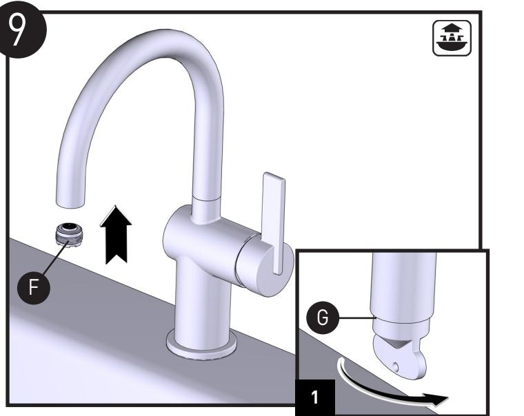
1. Reinstall Aerator (F) with Aerator tool (G).
