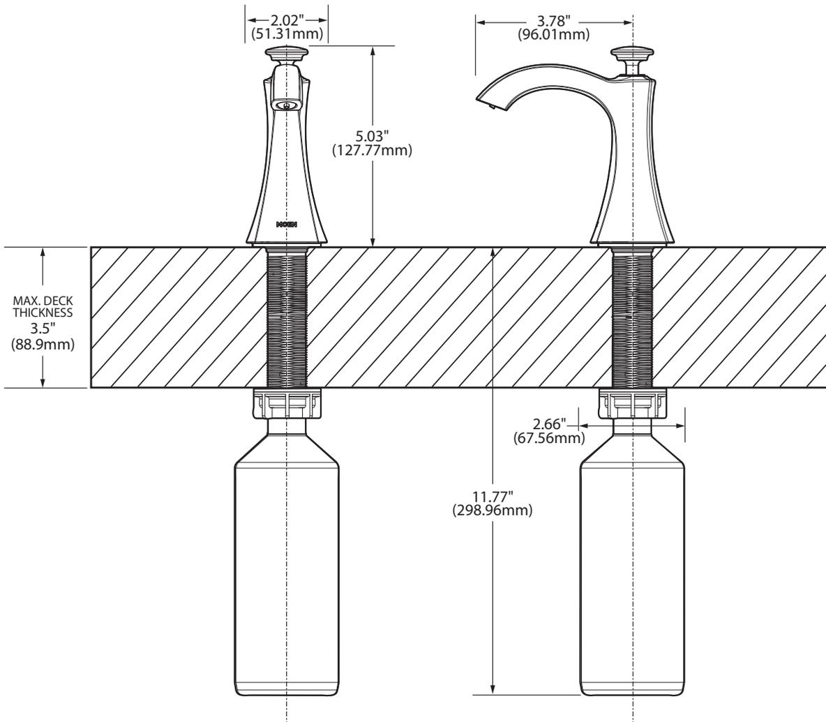
**NOTE:** DESIGNED TO BE INSTALLED THROUGH 1 HOLE 1-1/8" DIAMETER
