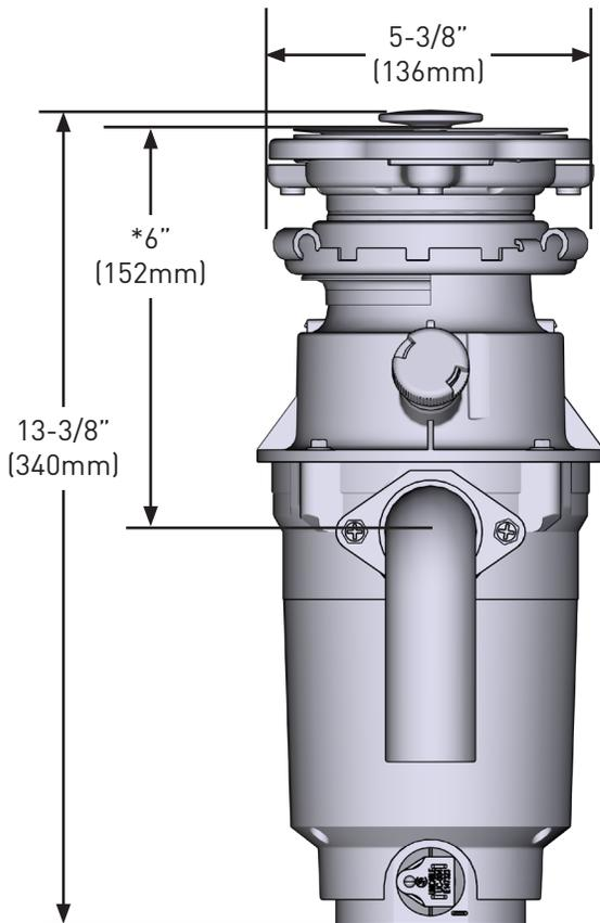
\*NOTE: Distance from bottom of the sink to center line of disposal discharge. Add 1/2" (13mm) when a stainless steel sink is used.
