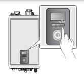
To turn the boiler on, press the Power button (心).
