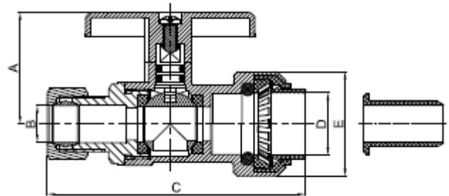
**Specifications:** Designed for residential, commercial or industrial use with water, specifically for use in copper, PEX, and CPVC systems. This valve features a fully removable grip assembly, ideal for use in potable water and hydronic heating systems.
