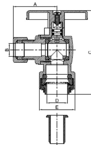
**Specifications:** Designed for residential, commercial or industrial use with water, specifically for use in copper, PEX, and CPVC systems. This valve features a fully removable grip assembly, ideal for use in potable water and hydronic heating systems.
