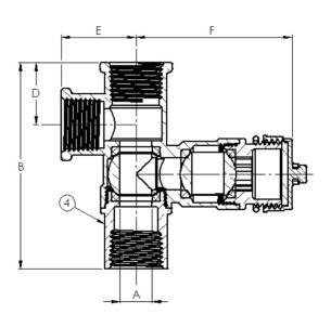
Designed for residential or light commercial use with water or oil. This approved Webstone valve allows for isolation and draining of an expansion tank in a closed loop hydronic heating system. It is actuated by a blowout proof stem and features an adjustable packing gland. Threaded ends comply with ANSI B1.20.1.
