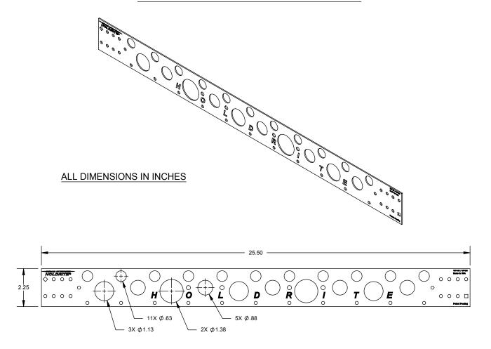
The HOLDRITE #107-26 is a Copper-Bonded™ steel bracket with holes for 1/2" tubings on 2" centers, holes for 3/4" tubings on 4" centers, holes for 1" tubings on 8" centers, and holes for 1-1/4" tubings on 8" centers.
