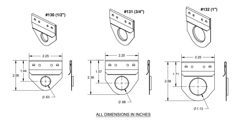
The HOLDRITE® #130, #131 and #132 are Solid Copper clips. Designed for easy snap-on installation for various flat strap brackets. 1/2", 3/4" or 1" copper tubes solder directly to the clip.
