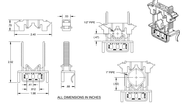
The HOLDRITE® Flame Fighter™ #250-S is a flame and smoke rated variable closure clamp compatible with Copper, PEX, CPVC tubing, conduit, etc. Supports up to 1" CTS tubing sizes. Material meets ASTM E-84 25/50 and UL94V-0 fire rating.
