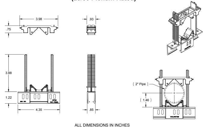
The HOLDRITE Stout Clamp™ #280-S is a flame and smoke rated variable closure clamp. Clamp supports 1" to 2" CTS/IPS tubing sizes. Supports Copper, PEX, CPVC tubing, conduit, etc. Material meets ASTM E-84 25/50 and UL94V-0 fire rating.
