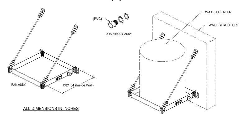
The Wall Mounted Equipment Platform is engineered to support water heaters up to 20 U.S. gallons (or other equipment up to 375 pounds total weight) mounted to a wall. This item also serves as a drain pan. See Installation Instructions for detail.
