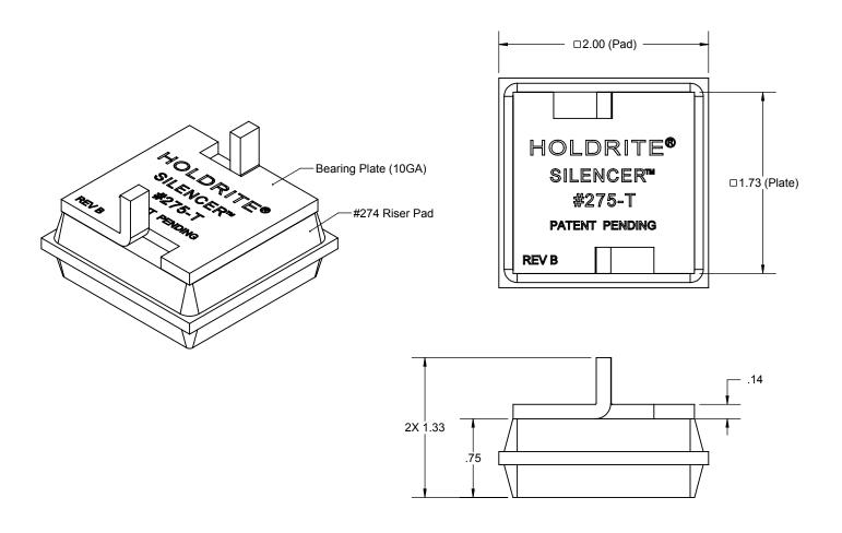
The HOLDRITE Silencer™ #275-T is an engineered noise and vibration isolating riser pad with a steel bearing plate. Ideal for use in isolating riser clamps from noise and vibration transfer to the structure. Unique vertical tabs protect from incidental displacement.
