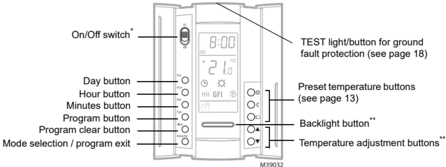
\* Place at Off to cut power to the heater (e.g., in the summer). This will not affect the time and temperature settings.
