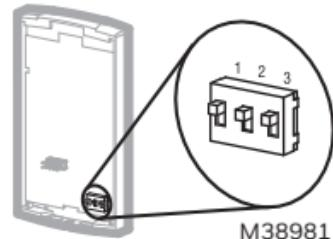
1. Early Start is used in Automatic mode only. When Early Start is enabled (on), the thermostat determines when to start heating so the Comfort temperature is attained at the beginning of periods 1 and 3. When Early Start is disabled (off), heating starts only at the beginning of periods 1 and 3; thus there is a delay before the Comfort temperature is reached.
