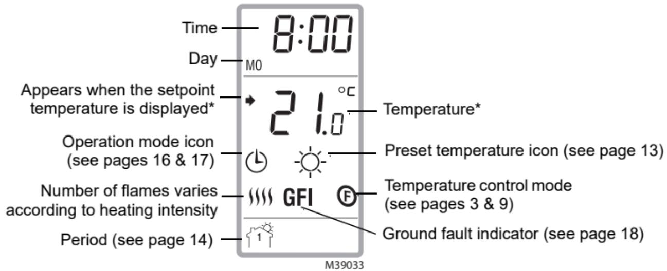
\* The thermostat normally displays the actual (measured) temperature. To view the setpoint temperature, briefly press either of the **▲▼** buttons. The setpoint will appear for 5 seconds. To change the setpoint temperature, press one of the **▲▼** buttons until the desired temperature is displayed. To scroll faster, press and hold the button.
