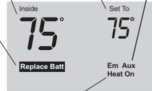
If "Heat On" or "Cool On" is flashing, compressor protection is engaged.
