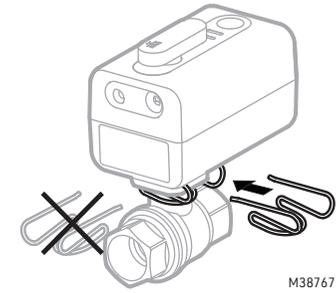
Fig. 4. Connect ball valve to actuator.
