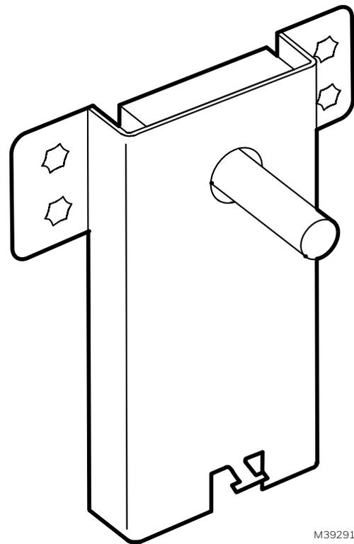
**Figure 8.** Anti-Rotation Slot Designation
