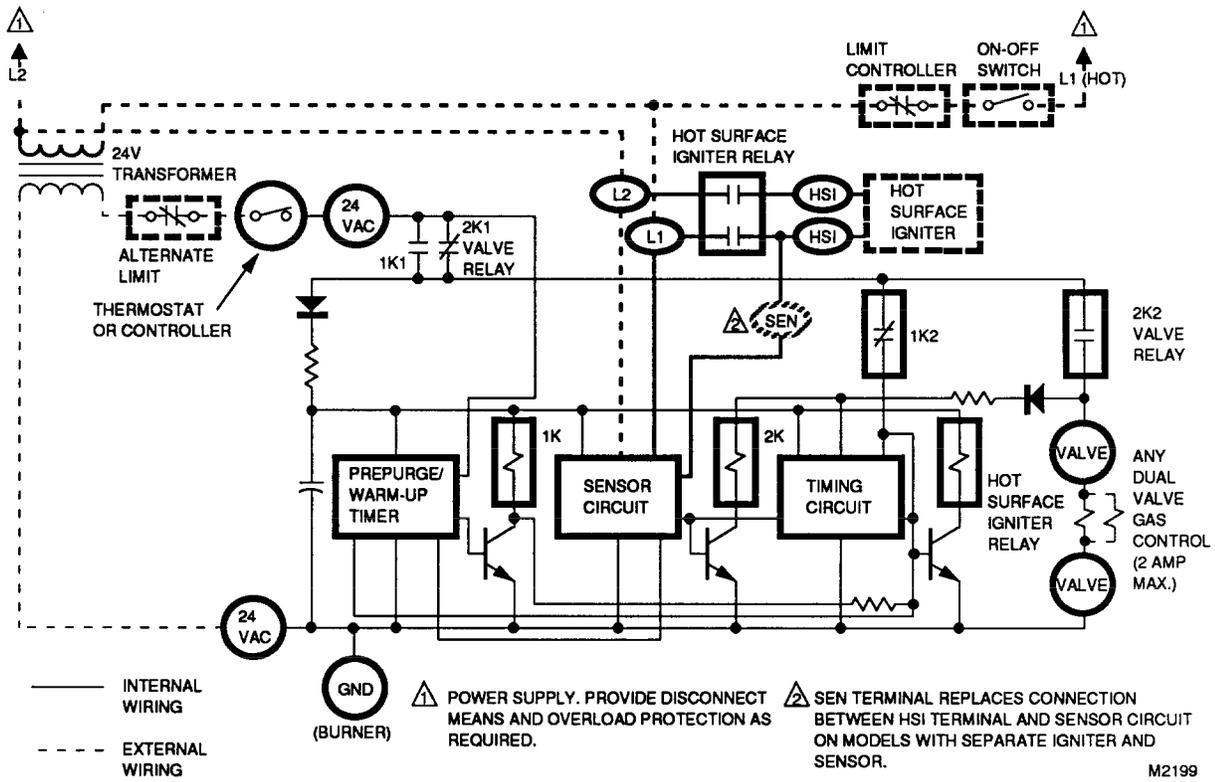
Fig. 14. S89/S890 simplified schematic.
