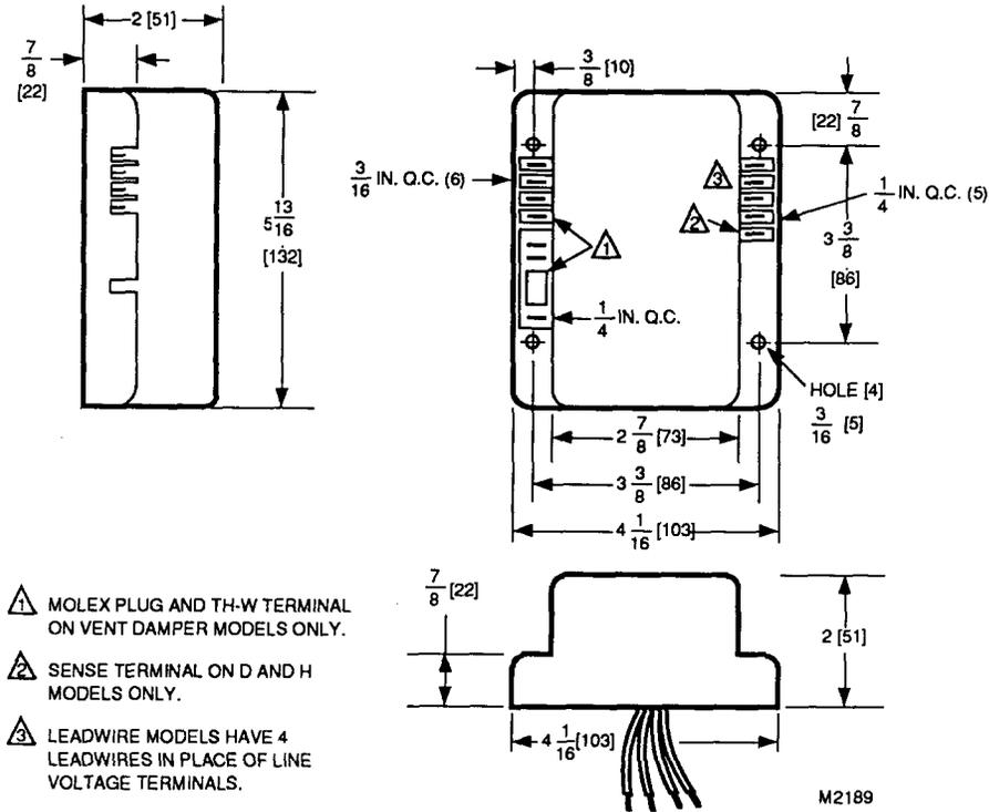
Fig. 1. Approximate S89/S890 dimensions in in. [mm].
