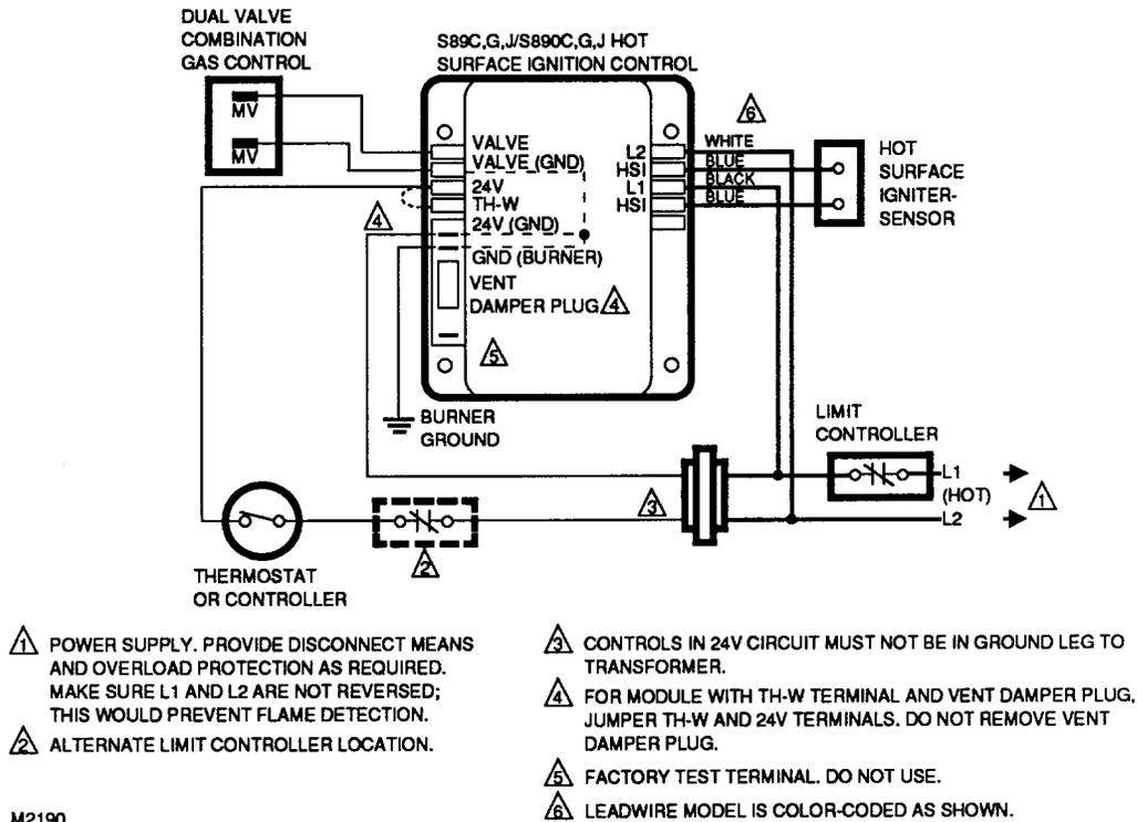
Fig. 2. S89C, G, J and S890C, G, J in an atmospheric burner heating system.
