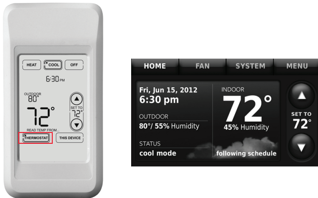
Fig. 312. Reading temperature at the thermostat.
