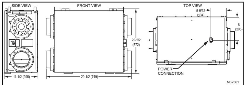
Fig. 1. Dimensions in in. (mm) and clearances.
