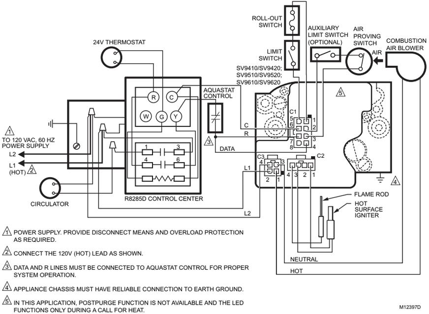
Fig. 9. SV9510/SV9520 typical boiler wiring diagram.
