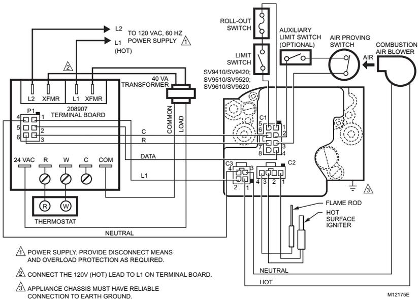
**Fig. 8. SV9510/SV9520 typical wiring connection with 208907 Terminal Board.**
