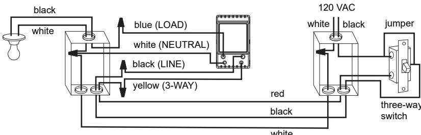
Connect the LOAD wire on the TI072 to the "common" wire, which you identified when removing the old switch. Connect the NEUTRAL wire to the neutral (white) wires. Connect the LINE and 3-WAY wires to the two remaining wires. At the other 3-way switch, connect the jumper wire between the "common" screw and the screw where the LINE wire of the TI072 is connected.
